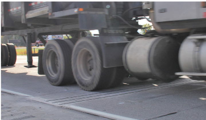
VectorSense™ Tire Sensors provide accurate axle classification
