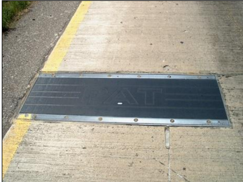
Figure 11 IRD PAT Bending Plate Weigh-in-Motion Scale
