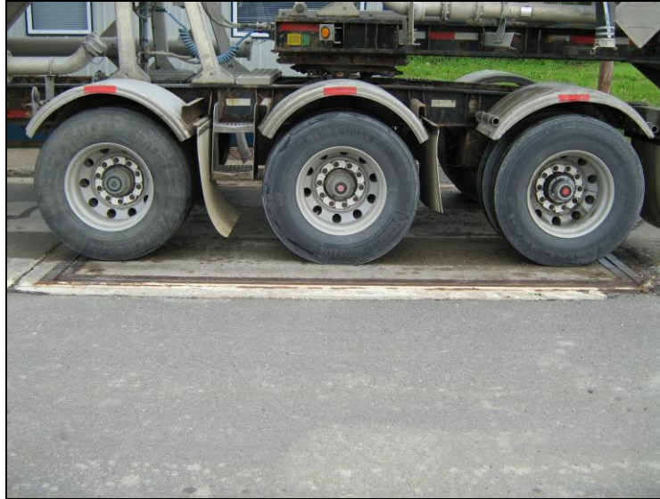
Figure 4 Commercial vehicle being weighed on Static Scale
