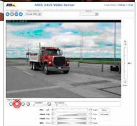
is viewed through an internet connection to an RCWS site. Multiple web browser windows allow the operator to view the monitoring sites, live video camera display, and static scale interface.
