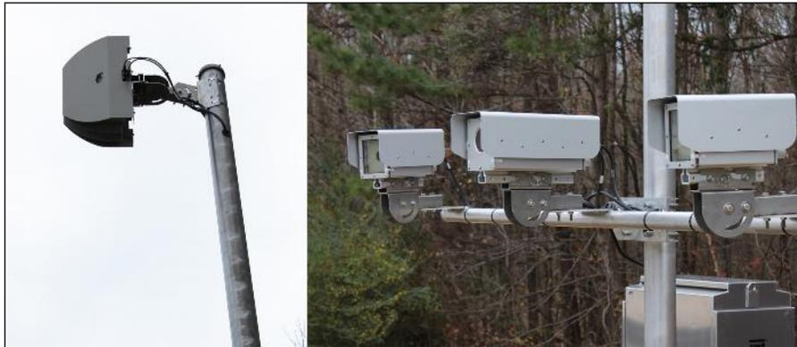
**Figure 4 – Laser Trigger (left) and HAZMAT Placard Camera and Illuminators (right)**
