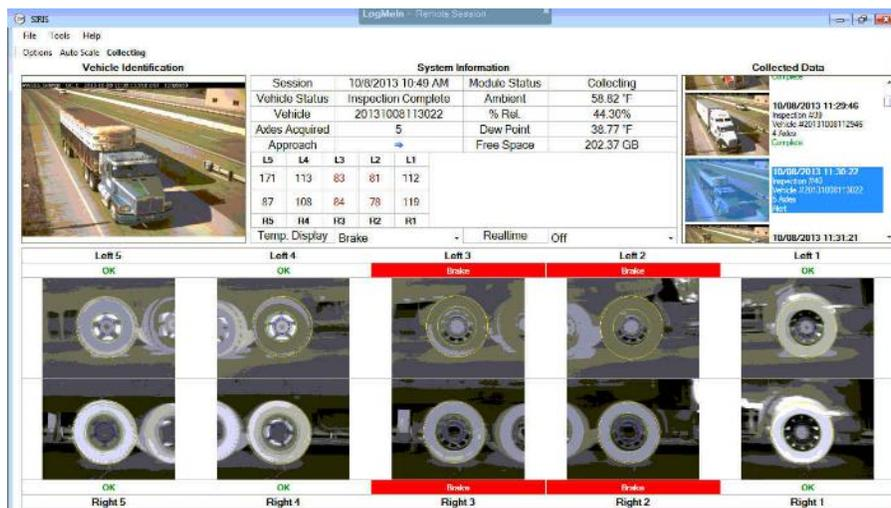
**Figure 6 – Automated Thermal Imaging System: Low Temperature Brake Alert**
