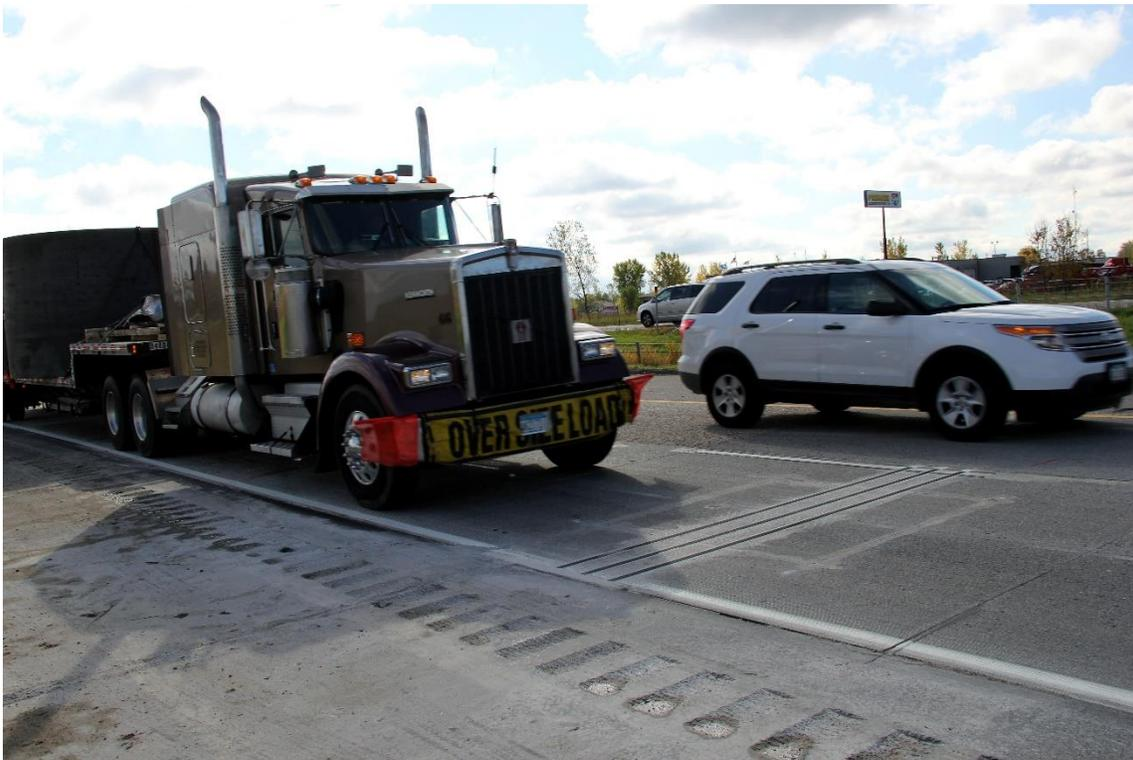
**Figure 1 – In-Road Tire Sensor Test Installation**
