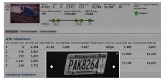
IRD's WIM scales and sensors are designed to accurately capture and record vehicle classification, speed, axle weights and gross vehicle weights as vehicles travel across the WIM location. This makes the weighing process more efficient, and in the case of commercial vehicles, it also allows for the pre-screening of overloaded vehicles at bridges.
