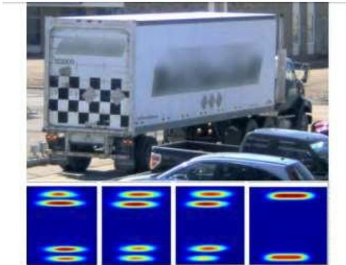
Figure 4 2D plot of Tire Pressure for a 4 Axle Truck
