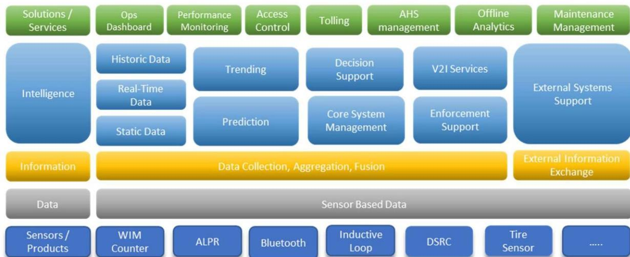
Figure 3 Central Data Collection System in the Context of Truck Mobility
